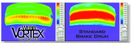
These photos taken from an infra-red camera mounted on the Webb dyno show a Webb Vortex® Unlimited drum next to a standard drum at precisely the same moment during braking. Compare the heat (red color) and you can actually see that Webb Vortex® Unlimited brake drums run significantly cooler.
