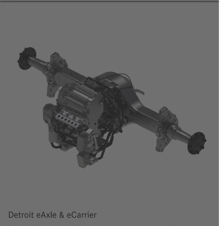
The Detroit eAxle integrates the function of the engine brake, drive axle and transmission into a drive unit with a reduced package size to optimize chassis space. Designed specifically for the eCascadia and eM2 products.
